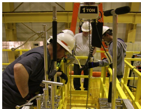
(Left) At MASF, workers practice with long-reach tools that will be used to retrieve sludge from the K West Basin. (Right) Workers deploy sludge retrieval tools at the actual reactor.
