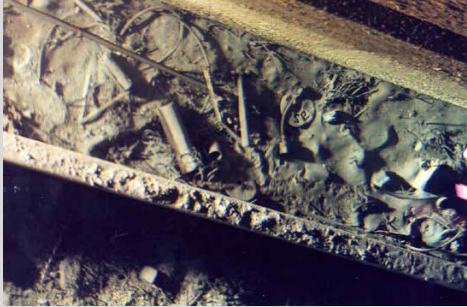
Sludge is a mixture of tiny fuel corrosion particles, fuel rod and metal fragments and soil and sand less than 1/4 inch (6 millimeters) in diameter.
