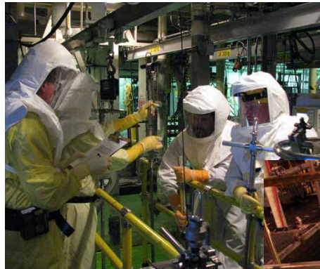
Workers (Above) use long-reach tools to access engineered containers that contain sludge in the basin (Right).
