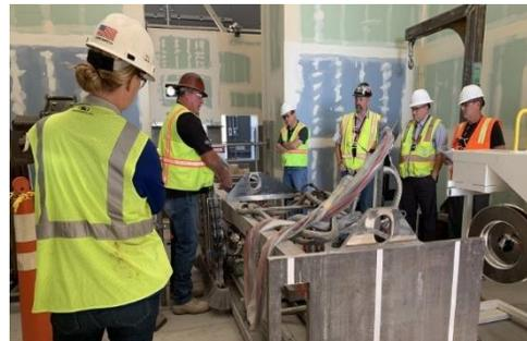
Workers installed and tested a saw at the mock-up, which will soon be installed in B Cell to cut through the concrete floor.
