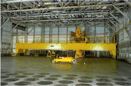
A yellow crane inside the 42,000 square foot Canister Storage Building is used to lift multi-canister overpacks from below-grade concrete vaults.
