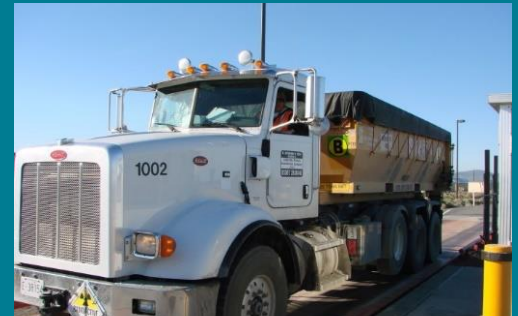
Environmental Restoration Disposal Facility containers are weighed and characterized to track waste contents.
