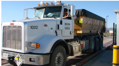
ERDF containers are weighed and characterized to track contents of waste.
