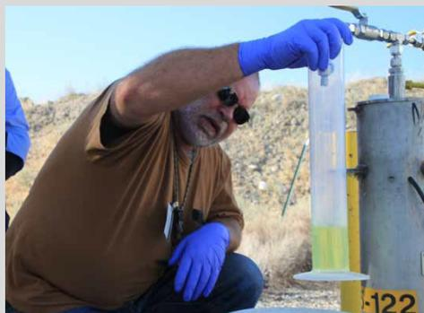
Groundwater containing hexavalent chromium being sampled from wells along the Columbia River.
