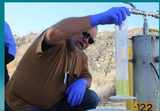
*Groundwater containing hexavalent chromium is sampled from wells near the Columbia River.*
