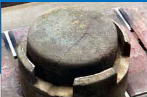
A plutonium "button" produced at Hanford's Plutonium Finishing Plant during production.
